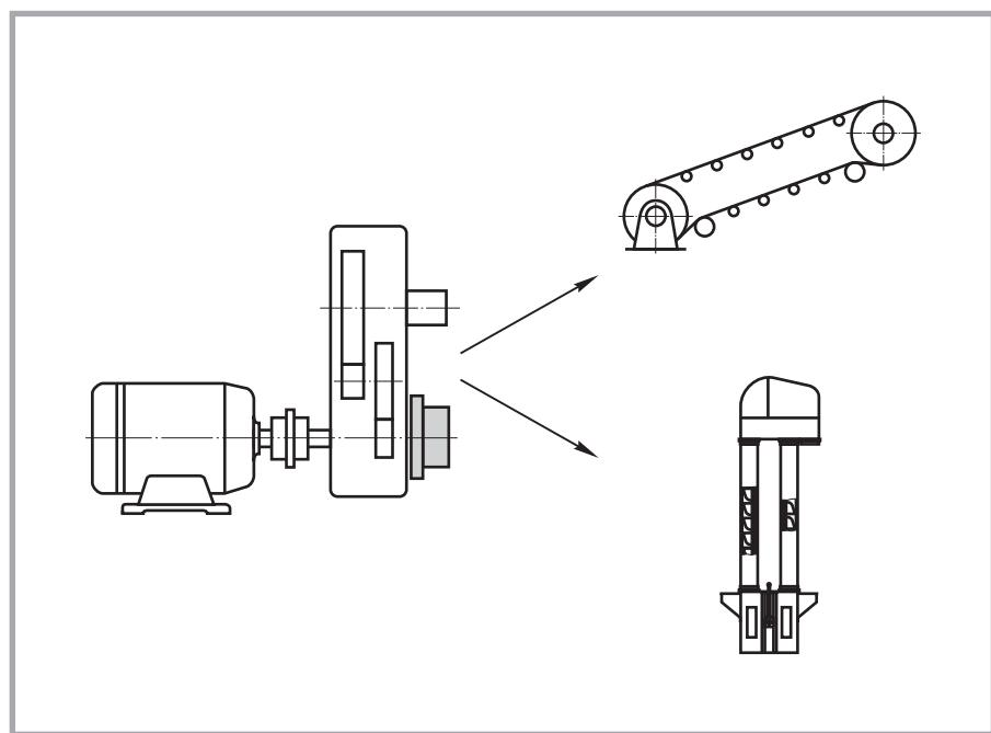
The backstop prevents reverse rotation of the conveyor belt or elevator in case of a power failure or when the motor is turned off.
