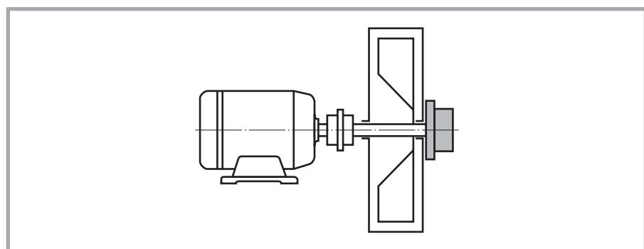
The backstop prevents reverse rotation in case of fluid backflow.
